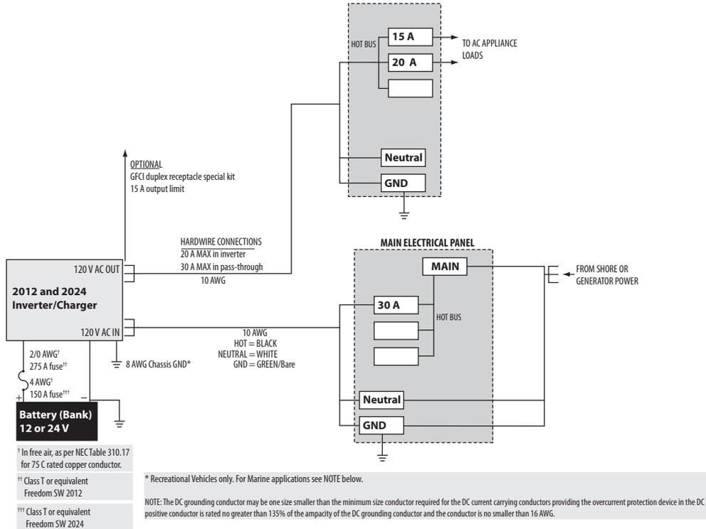
**IMPORTANT:** Read Owner's and Installation Guides prior to installation. Always refer to local and national electrical codes for proper wire and breaker sizes prior to installation.
