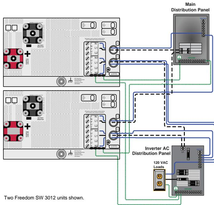
**Figure 17** Parallel Stacking Using Two Freedom SW 3012s
