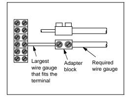
Note: The maximum wire size that the connectors bear is of 6AWG. If the wire gauge must be larger, have the installation carried out by specialized personnel, using adapter connectors, as shown above.
