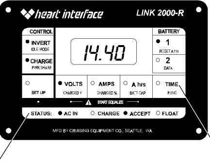
Status lights indicate which cycle the regulator (and /or the charger) is in. The AC light will be <u>OFF</u> if there is no external AC input. Selecting TIME when the alternator regulator is operating displays the alternator output current. The current is displayed with an "A " preceding the value.
